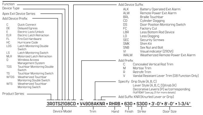
**DEVICE ONLY:** List quantity, device model w/function, hand, finish, strike, and door size including thickness. Note: For greater exit device mounting heights, see extended bottom rods (pages 35, 36, 37 & 38)
